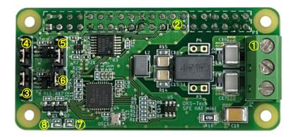
1. Single pair Ethernet cable and shield wire connection terminal
